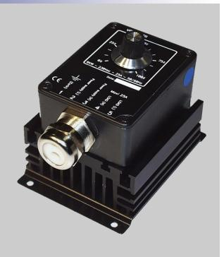
autonomous and compact AC energy regulator for proportional linear control of resistive load using bust fire control (load with high inertia) or using phase angle variation (load with low inertia). Can be used with most resistance heaters.
