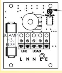
CAUTION: Use insulated trimmer to adjust cermet for required duty cycle.
